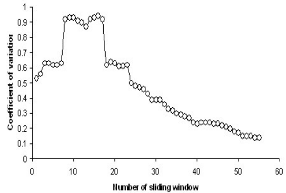
Fig. 3. Coefficient of variation of power of acoustic emission time series at increased external forcing for 500 data length sliding window with 50 data shift. Here only half of record of Fig.1 is used from the start of the test to the maximum synchronization state.
